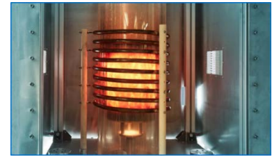
Figure 1: sublimation growth reactor T > 2000^{\circ}\text{C}
